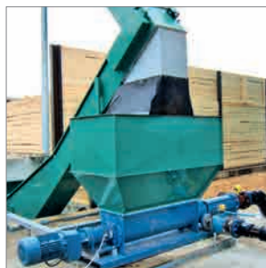
Feeding the pump via a transferring hopper
