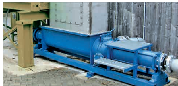
Introduction of solid substances after crushing
